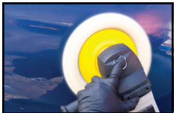
Spread the product on the surface and compound at 1500 - 1800rpm
