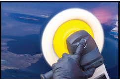
Using minimal pressure, compound at 2000 - 3500rpm
